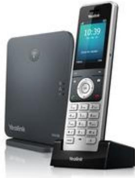
The Yealink W60P SIP cordless phone system combines quality, reliability and flexibility to offer users a scalable, efficient communications system. With support for up to 8 W52H/W53H/W56H handsets and up to 8 concurrent calls, the W60 features upgraded firmware and a range of features including call hold, call transfer, 3-way conferencing and support for Opus audio codec.
