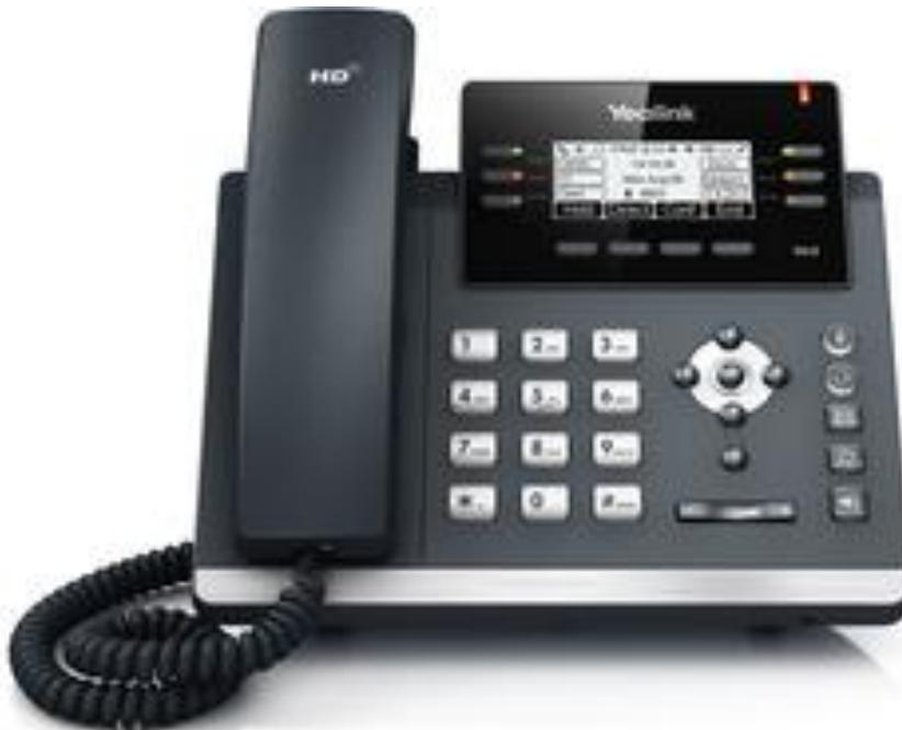
Yealink's new T41S marks the entry level model in the new T4S Series. Ideal for business users, the T41S delivers superb audio quality as well as a rich visual experience with a 2.7" graphical LCD screen and support for up to 6 SIP accounts.
