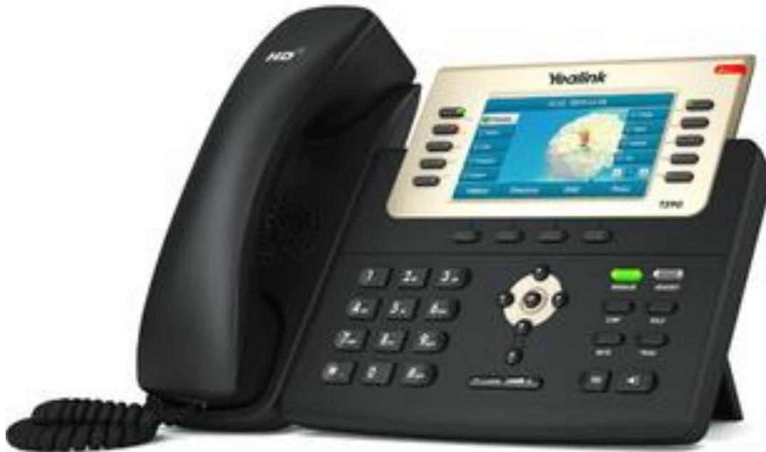
The T29GN is an executive IP phone which supports up to 16 SIP accounts and has a built in two-port Gigabit Ethernet switch. This phone offers a high resolution TFT colour display and Optima HD technology delivering a rich visual and audio experience along with a very user friendly interface. There is support for corded, Bluetooth (requires BT40) or wireless/DECT headsets supporting EHS (requires EHS36 adaptor).
